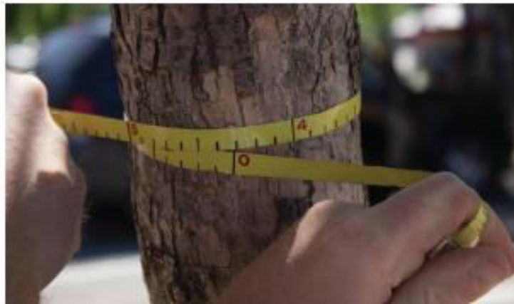
The correct diameter measurement is 4.3, when reading from right to left.
